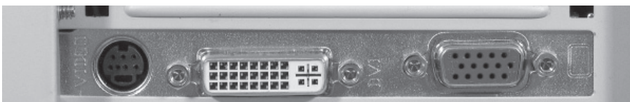
Figure 2-24 Video card with three ports. From left to right, S-Video, DVI, and VGA.
