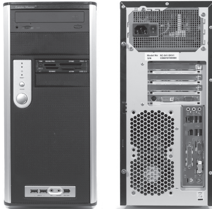
Figure 2-36 Front and back of a typical PC case showing various buttons and ports
